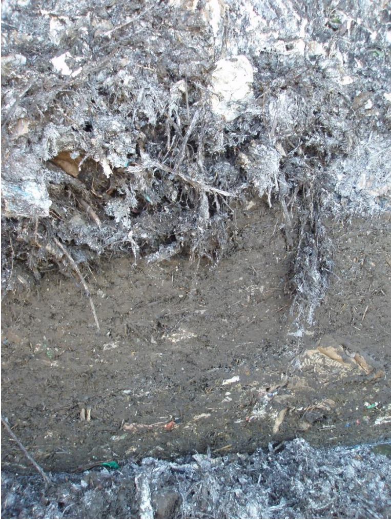
Figure 2: Densely packed material and poor diffusion of gases
