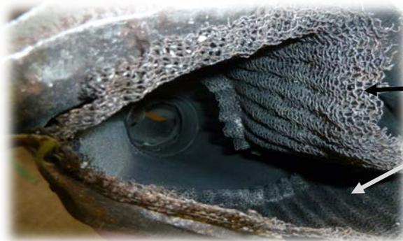
Metal mesh matting in a catalytic converter without RCF matting
