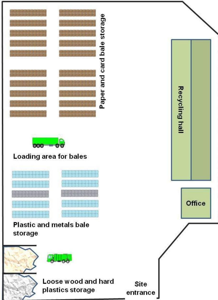
**Example: Material recycling facility producing baled paper, plastics and metals, plus loose hard plastics and wood.**
