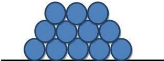
Round/tubular bales and loose materials which may roll should a stack collapse during a fire may result in fire spread – such factors need to be taken into account in your calculations to arrive at separation distances
