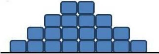
Pyramid/terraced storage of bales may lessen the risk of a bale falling during a fire resulting in fire spread. However, this method may increase bale footprint relative to volume and may cause operational handling issues
